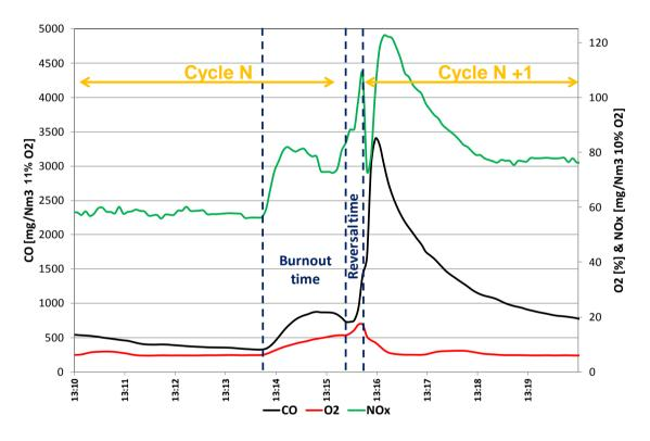
Figure 1: Detail of the emissions during kiln reversal
